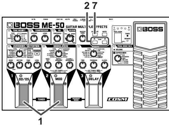
1. Press the number 1 and 2 pedals simultaneously to switch to Tuner mode.
