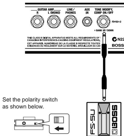
By connecting with a special cable (the optional PCS-31), you can connect two foot switches, and use them to switch Banks up and down.
