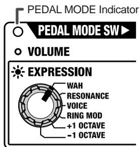
You can make the setting that determines whether the ME-50's expression pedal functions as a volume pedal or as an expression pedal. In addition, when using it as an expression pedal, you can use it to control one of the special pedal effects that you select.
