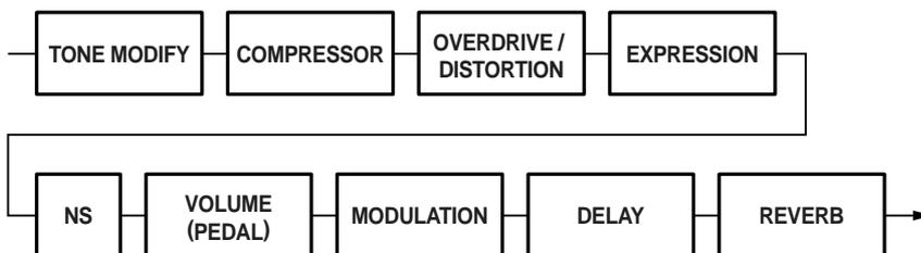
Also, when the MODULATION type is TREMOLO or UNI-V, MODULATION is connected before OVERDRIVE/DISTORTION.
