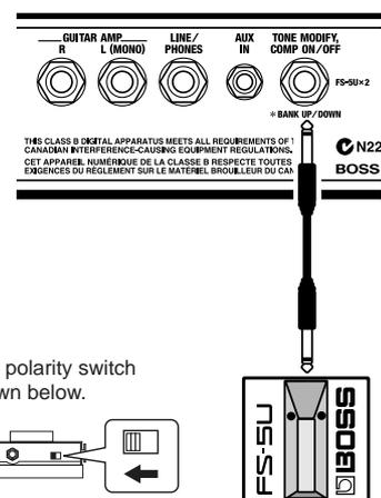
Set the polarity switch as shown below.
