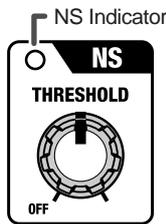
This effect reduces the noise and hum picked up by guitar pickups. Since it suppresses the noise in synchronization with the envelope of the guitar sound (the way in which the guitar sound decays over time), it has very little effect on the guitar sound, and does not harm the natural character of the sound.
