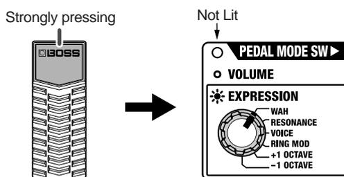
The volume decreases as the pedal's toe is raised, and increases when the pedal is pressed down.
