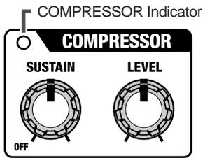
This is an effect that produces a long sustain by evening out the volume level of the input signal. You can also use it as a “limiter” to suppress only the sound peaks and prevent distortion.
