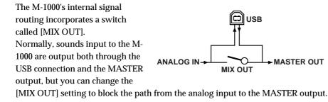
When using the M-1000 in combination with another mixer, the way the connections are made and the mixer is structured can cause sounds to be output twice. This occurs in the following cases.
