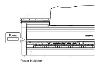
To turn the power off, turn the [Volume] knob all the way to the left, and press the [Power] switch.
