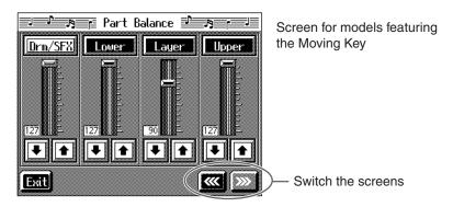
This shows the volume balance between the keyboard's Tones when either layer performance (p. 30) or split performance (p. 31) are used, or the volume balance when using the keyboard to play percussion instruments or sound effects (p. 28).
