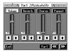
You can change the Tone for the selected Part by pressing a Tone button while this screen is displayed. When selecting Part 10 or 11, you can touch <Drum Set> to select the drum set or effect sound.
