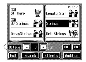
**4.** Touch Octave <-> or <+> in the lower part of the screen to adjust the pitch of the sound.
