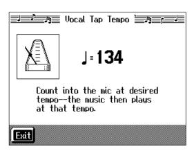
**4.** Count to four ("One, two, three, four") into the mic.
