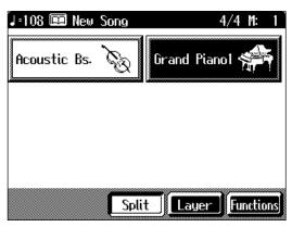
The tone sounding prior to the split performance is played in the right-hand section of the keyboard, and the tone indicated at the left of the screen is played in the left-hand section of the keyboard.
