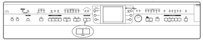
When the Basic screen is displayed, you can use the Tempo [-] [+] buttons or the [-] [+] buttons and the dial to change the tempo.
