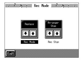
**3.** Touch <Rec Stop> to switch between "Arranger Stop" and "Composer Stop."
