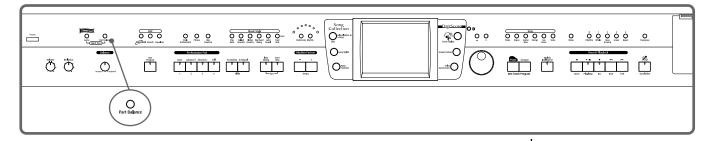
**1** • Press the [Part Balance] button and watch the indicator light up.
