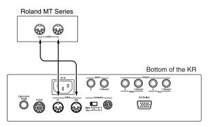
\* When the KR is connected to a MIDI sequencer, set it to Local OFF. Refer to "Disconnecting the Keyboard from the Internal Sound Generator (Local On/Off)" (p. 174).
