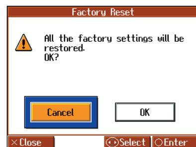
2. Press the cursor right button to select <OK>, then press the [ O ] button; the Factory Reset is executed. Once the Factory Reset has been completed, switch the power off, then on again.
