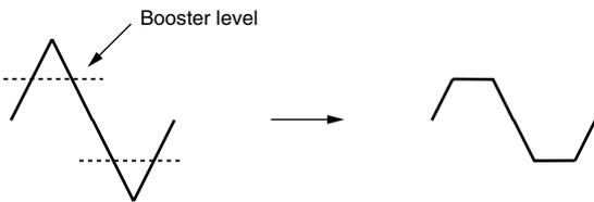
In addition to using this to create distortion, you can use the waveform (WG1) of one of the tones as an LFO which shifts the other waveform (WG2) upward or downward to create modulation similar to PWM (pulse width modulation). This parameter works best when you use it in conjunction with the Wave Gain parameter (p. 54).
