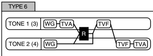
This type uses a ring modulator to create new overtones, and in addition mixes in the sound of tone 2 (4) and stacks the two filters. Since the ring-modulated sound can be mixed with tone 2 (4), tone 1 (3) TVA can adjust the amount of the ring-modulated sound.
