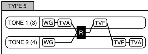
This type uses a ring modulator to create new overtones, and combines the two filters. The tone 1 (3) TVA will control the volume balance of the two tones, adjusting the depth of ring modulator.
