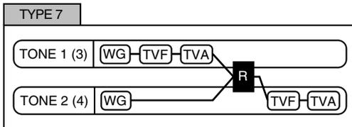
This type applies a filter to tone 1 (3) and ring-modulates it with tone 2 (4) to create new overtones.
