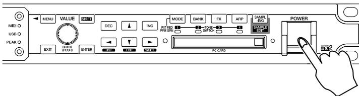
\* This unit is equipped with a protection circuit. A brief interval (a few seconds) after power up is required before the unit will operate normally.
