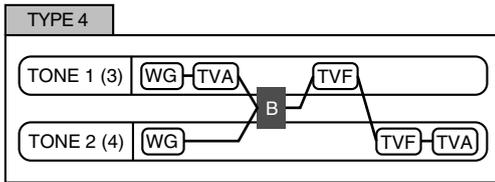
This type applies a booster to distort the waveform, and then combines the two filters. The TVA for tone 1 (or 3) controls the volume balance between the two tones and adjusts booster level.
