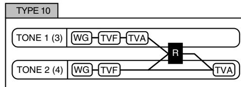
This type passes the filtered sound of each tone through a ring modulator to create new overtones, and also mixes in the sound of tone 2 (4). Since the ring-modulated sound can be mixed with tone 2 (4), tone 1 (3) TVA can adjust the amount of the ring-modulated sound.
