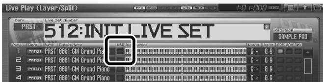
2. Press [INC] to turn on the keyboard switch for part 1.
