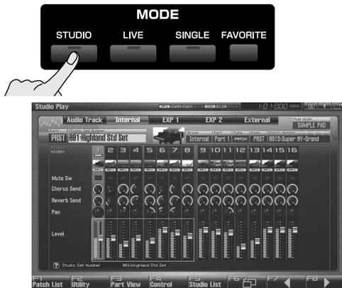
In Studio mode you can use up to sixteen sounds to play a different instrument for each part, so this is the ideal mode for playing a song that uses an ensemble of multiple instruments such as drums, bass, and piano.
