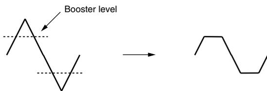
In addition to using this to create distortion, you can use the waveform (WG1) of one of the tones as an LFO which shifts the other waveform (WG2) upward or downward to create modulation similar to PWM (pulse width modulation). This parameter works best when you use it in conjunction with the Wave Gain parameter (p. 92).
