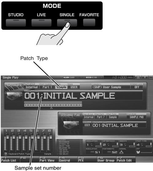
\* Make sure that the Patch Type is set to "Sample." If this is set to "Patch" or "Rhythm," use [CURSOR] to move the cursor to the patch type, and turn the VALUE dial or press [INC] [DEC] to select "Sample."
