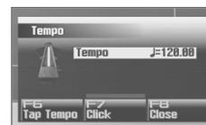
2. Turn the VALUE dial or use [INC] [DEC] to specify the tempo. By holding down [SHIFT] while you turn the VALUE dial, you can adjust the value below the decimal point.
