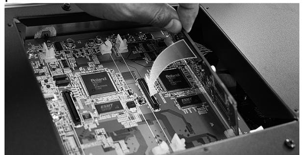
\* Never use excessive force when installing a circuit board. If it doesn't fit properly on the first attempt, remove the board and try again.
