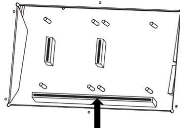
3. **Press outward on the white clips at either end of the socket so they are in their downward position.**
