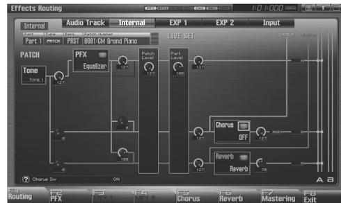
2. Use [CURSOR] to move the cursor to the switch for each effect, and turn the VALUE dial or use [INC] [DEC] to turn the switch on/off.
