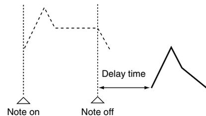
**OFF-D:** Rather than being played while the key is pressed, the tone begins to play once the period of time specified in the Delay Time parameter has elapsed after release of the key. Here, however, changes in the TVA Envelope begin while the key is pressed, which in many cases means that only the sound from the release portion of the envelope is heard.
