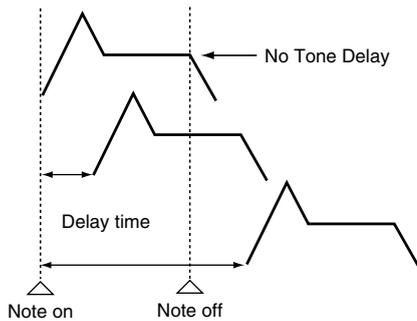
**HOLD:** Although the tone begins to play after the time specified in the Delay Time parameter has elapsed, if the key is released before the time specified in the Delay Time parameter has elapsed, the tone is not played.
