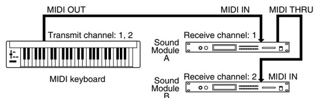
When used as a sound module, the Fantom-G can receive on up to sixteen MIDI channels. Sound modules like the Fantom-G which can receive multiple MIDI channels simultaneously to play different sounds on each channel are called **multi-timbral sound modules**.
