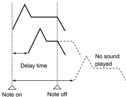
**OFF-N:** Rather than being played while the key is pressed, the tone begins to play once the period of time specified in the Delay Time parameter has elapsed after release of the key. This is effective in situations such as when simulating noises from guitars and other instruments.
