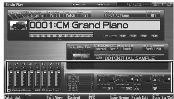
2. While playing the keyboard to produce sound, operate the knobs, sliders or [S1] [S2] buttons.
