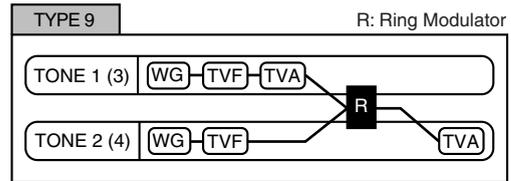
This type passes the filtered sound of each tone through a ring modulator to create new overtones. The tone 1 (3) TVA will control the volume balance of the two tones, adjusting the depth of ring modulator.
