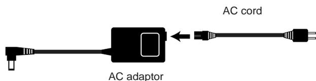
2. Connect the AC adaptor to the DC In connector on the rear panel.
