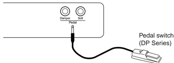
When connected to the Damper jack, the pedal can be used as a damper pedal.
