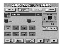
Press the field of the parameter you want to edit and use the <u>DATA/ENTRY</u> dial or the <u>DEC</u>/<u>/INC</u> buttons to set the desired value. You can also press the <u>DATA/ENTRY</u> dial and use the numeric pad.
