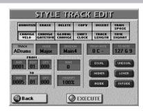
The CHANGE VELO function allows you to modify the dynamics (called "velocity") of a track or excerpt. See p. 135 for details. Only note events can be changed.
