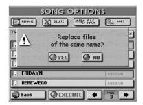
(7) Press the YES field if it is OK to overwrite files with the same names on the destination media. Press the NO field if files on the source ("FROM") media that have the same name as existing files on the destination ("TO") media should not be copied (only files with "original" names will be copied in that case).
