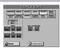
INSERT allows you to insert space and shift data that lie behind the FROM position further towards the end of the song (this is the exact opposite of DELETE). These empty measures can be "filled" using the COPY function or by recording new phrases in that area (using PUNCH IN/OUT, for example). (page 133).
