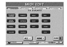
Press the <u>ALL</u> field to switch all button icons on (the corresponding messages are then transmitted). Press <u>NONE</u> to switch all button icons off. Press <u>CLOSE</u> to return to the page where you came from. You can also switch the following button icons on/off individually:
