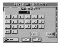
Here, you can either set the required length as a CPT value ( $\downarrow$  = 120CPT) or use the note fields to avoid lengthy calculations. Use the numeric pad to enter the desired duration. Drum parts usually use the Gate Time value "1" for all notes. Increasing it to "20", for example, has no audible effect on the sound durations. The maximum duration a note event can have is 99,999 clocks, which corresponds to roughly 208 bars.
