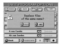
(6) Press the  $\boxed{YES}$  field if it is OK to overwrite files with the same names on the destination media. Press the NO field if files on the source ("FROM") media that have the same name as existing files on the destination ("TO") media should not be copied (only files with "original" names will be copied in that case).
