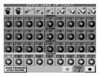
(The difference between these two pages is that the "USER PROGRAM..." settings can be saved to a User Program, and are therefore "temporary" modifications of the Style data, while the "STYLE MAKEUP TOOLS" settings can be "burned" into the Style itself.)
