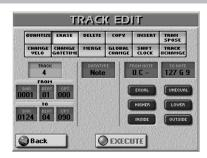
ERASE allows you to selectively delete data either within a specified range of measures, beats or clocks or from the entire track(s). When DATA TYPE is set to "ALL", ERASE substitutes the required number of rests for the data you delete, so that you end up with the equivalent number of blank measures. If you also want to eliminate the measures themselves, use DELETE (see below).
