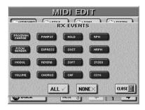
The RX events are the same as the TX events, except for the "CAF" parameter (reception of Channel Aftertouch messages), which can be received – or filtered. Press the Back field and save your settings to a MIDI Set; -or-
