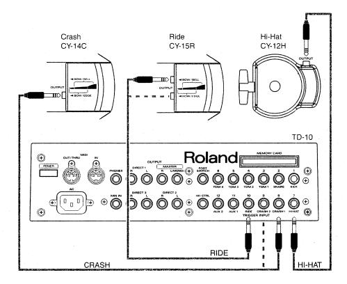
Use the supplied connection cables (stereo) to make the connections. If monaural cables are used, edge shots, bell shots, and choke play cannot be supported.
