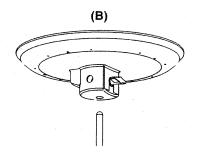
There are two ways to use the drum stand mounting rod. Before changing how the rod fits, fixing screw, then turn the inner bolt 90 degrees.
