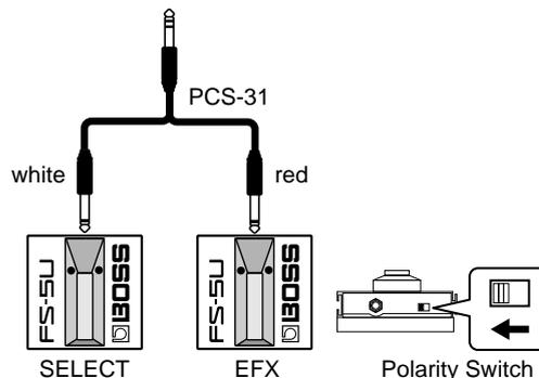
\* *When you connect only one foot switch by mono cable, you can only use it to switch channels (JC CLEAN/LEAD).*
