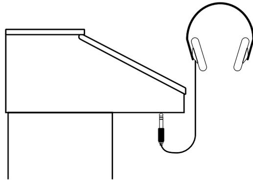
1. Connect the headphones to the Phones jack on the underside of the unit.
