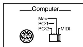
\* When the AT-20S is powered up, the setting doesn't change until the power is reset, even if the computer switch is operated.
