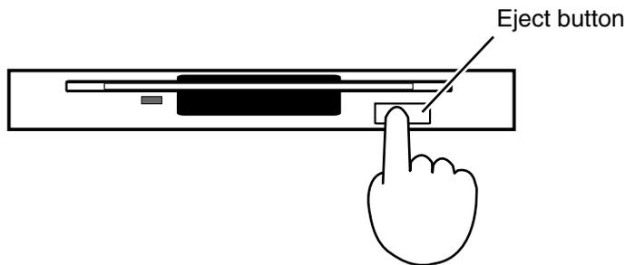
The floppy disk is ejected a little out of the slot. Gently grasp the end of the floppy disk and pull it out.
