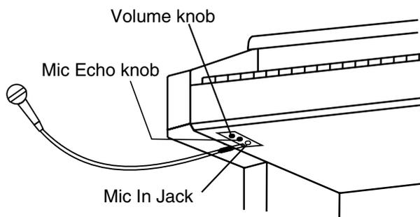
1. Connect a microphone (sold separately) to the Mic In jack on the lower-right area of the instrument.
