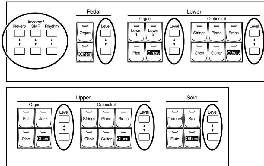
The following buttons are used to adjust the volume of a multiple number of Parts.
