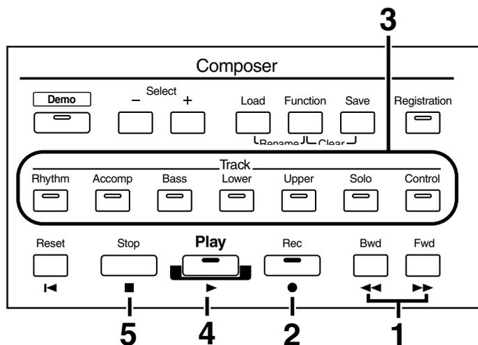
**1.** Press the [Reset] button or the [Bwd] / [Fwd] buttons to move to the measure (bar) where you wish to start re-recording.
