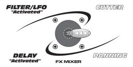
To fade-in one effect before the other, move the joystick around the edge of the aperture towards the preferred effect and then inwards to bring in the second effect.
