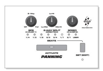
This part of the FEDERATION is quite revolutionary. There have of course been auto-panning devices before, which could use an LFO to move a signal around the stereo field, but none which could trigger this LFO from a BPM analyser and certainly none which could move different frequency bands to different pan positions at the same time.
