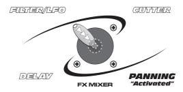
**Example 2 - Fade-In/Out the FILTER/LFO and DELAY effects:** Position the joystick over to the right, in between the CUTTER and PANNING positions as shown below and ensure all effects are de-activated. Activate the FILTER/LFO and DELAY effects and then select the MASTER to ON. The audio track will be un-effected until the joystick is moved away from the mid CUTTER/PANNING position. To fade-in both effects simultaneously, move the joystick in a straight line towards the centre position.
