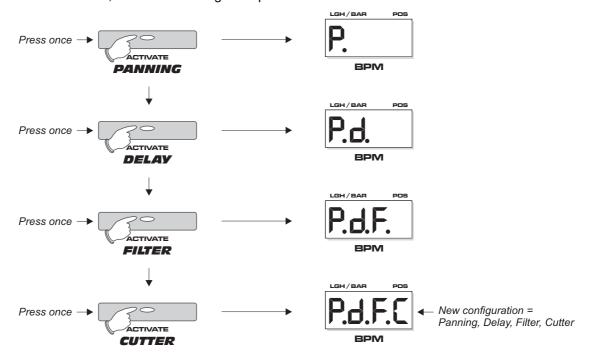
Effects cannot be entered twice. After all four effects have been entered correctly, the operating system will automatically exit Utility mode.
