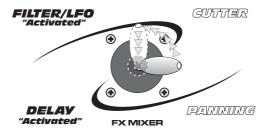
At the central 'upright' position, the level of both effects will be at their maximum i.e. moving the joystick past the upright position towards the FILTER/LFO or DELAY positions will have no further effect.
