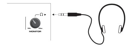
Slowly turn the MONITOR control clockwise until a comfortable level is reached. If no effects are activated, the unaffected audio signal alone will be heard.
