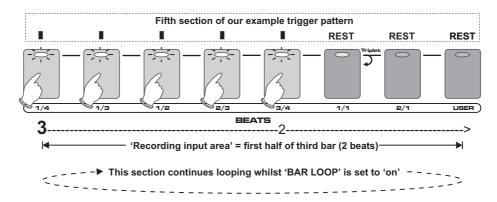
To exit 'BAR LOOP' mode simply press the 'BAR LOOP' button again (LED off). The pattern will now continue to play onwards from the end of the current loop section.
