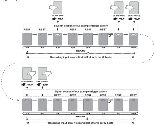
The quantize setting will automatically correct the timing of any trigger events you tap-in to the nearest set beat.
