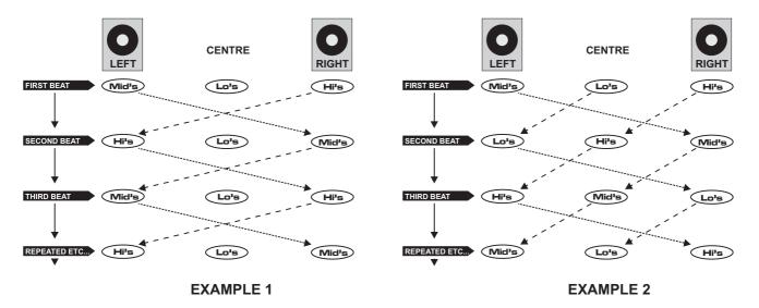
When the SET(EDIT) button is pressed and held down (LED flashing) this control sets the directional movement of Spatial Panning (when SPS is set to 'Full'). Between the fully anti-clockwise and 12 o'clock position the SPS movement will be RIGHT - to - LEFT. Between the 12 o'clock and fully clockwise position the SPS movement will be opposite, LEFT - to - RIGHT. The main BPM display will indicate the settings as follows:
