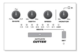
This effect operates in a similar fashion to the filter but on the overall volume of the signal. The cutter can be set to operate either as a conventional 'gate' which, each time it is triggered opens instantly to allow signal through but then after a short period closes completely to cut off the signal, or as a fade-in/fade-out control with a relatively short period of operation.
