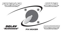
To mainly hear the PANNING effect, move the joystick to the South/East position, as in the following example:
