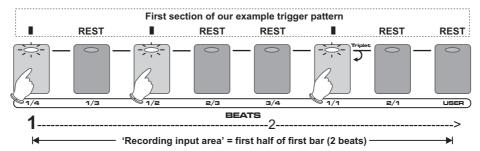
To remove an event, simply press the highlighted button(s) again and the indicator will go out. After showing the first 2 beats of the first bar, the BEATS buttons will show the second 2 beats of the bar, as in the following example:
