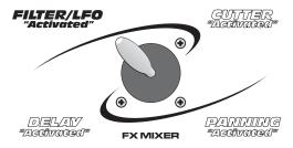
To mainly hear the CUTTER effect, move the joystick to the North/East position, as in the following example:
