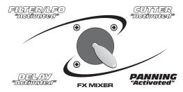
When the joystick is placed in a position other than those detailed above the result will be a unique blend of the activated effects. With all four effects activated, try moving the joystick around to get a feel of the variations possible. You can also use the FX MIXER to fade-in or fade-out one, two or three effects, as detailed in the following example:
