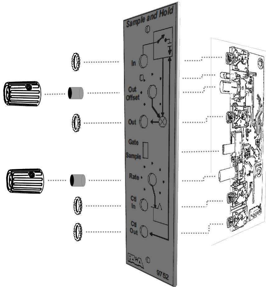
Fig. 1A Attach board to panel using connector nuts, shim control shafts, and rotate controls to minimum and tighten set-screw knobs to agree.
