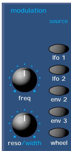
This is an extremely powerful feature of the Supernova II keyboard. These controls affect the modulation of the Filter. The knobs on the left are "Destinations". They can all be modulated by the "Sources" which are the buttons on the right. The amount of modulation applied from any source is determined by the setting of the knobs. This can be either positive modulation ( Turning either or both of the knobs Clockwise ) or negative modulation. ( Turning either or both of the knobs Anticlockwise )
