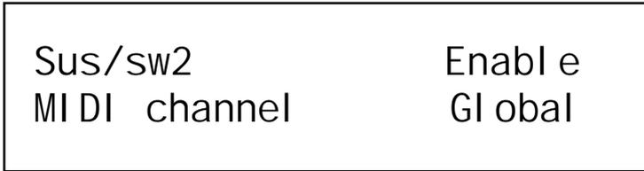
The "Sus/sw2" parameter on page 1 of the Midi Menu determines how the Part will respond to sustain MIDI messages (CC 64). These messages could be generated directly by a footswitch connected to the "Input / sw 2" jack or received from a sequencer via MIDI In. The options available allow a wide range of features from normal sustain operation to Arp latching, Arp muting etc. including inverted operation.
