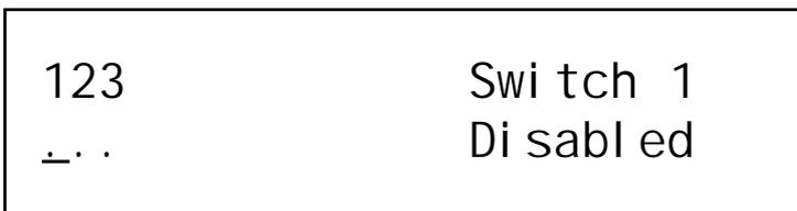
Page 4 in the Midi menu has a single parameter for each of the three pedal / switch jack sockets. This parameter determines whether pedal / switch MIDI data will be transmitted ( and passed on to the Part ). If the jack socket parameter is set to "Enabled" ( "o" ), then when the pedal / footswitch is moved, the appropriate MIDI data will be transmitted using the Part's own MIDI channel. This MIDI data will then be passed to the Part.
