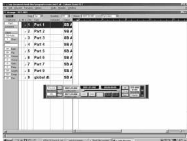
To play or edit the first Part in a multi-timbral Performance, select (highlight) the sequencer track corresponding to Part 1. Now select Part 1 on the Supernova II's front panel and change the Program assigned to Part 1 as you wish. The MIDI information transmitted by Part 1 is being re-routed back to the Supernova II Keyboard's MIDI channel for Part 1 (MIDI channel 1).
