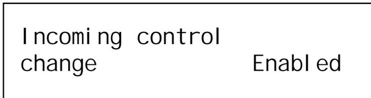
The parameter is "Incoming control change". In this case with a value of Enabled. This parameter determines if the Supernova II keyboard responds to incoming MIDI controller messages or not. Use the lower Data knob to adjust this parameter. This filter is global and applies to all playing modes. The range of this parameter is Enabled & Disabled. This parameter is memorised with the Global settings.
