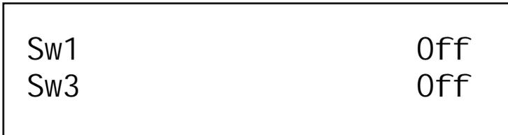
The "Sw 1" parameter on page 2 of the Midi Menu determines how the Part will respond to NRPN 9082 MIDI messages. These messages could be generated directly by a footswitch connected to the "Input / sw 1" jack or received from a sequencer via MIDI In. The options available allow a wide range of features from sustain operation to Arp latching, Arp muting etc. including inverted operation.
