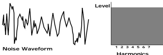
White noise has no fundamental and so all harmonics are the same value. This wave can be used by itself to synthesise explosions or wind, and when used in conjunction with other waveforms can be used to create the illusion of "Breath" in an instrument.
