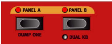
Both Panels activated. One of the **PANEL** button LEDs will blink to indicate which Panel is currently has edit focus.
