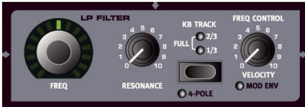
The filter is, together with the oscillators, the most important sound-shaping tool in a synthesizer. The filter section in Nord Stage comprises a lowpass filter with either a 12dB or 24 dB slope, with selectable keyboard tracking. The filter has adjustable resonance, and is self-oscillating at high resonance settings. The filter cut-off frequency can be modulated by velocity or by the Mod Envelope.
