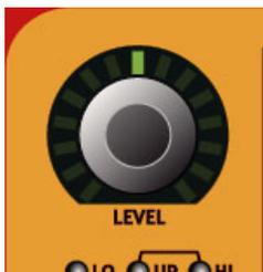
Each instrument has a **LEVEL** rotary encoder at the top. This adjusts the output level for the corresponding instrument section. The **LEVEL** encoders can be Morph controlled.
