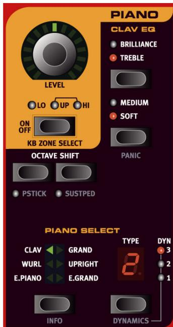
The Piano section of Nord Stage contains six Piano Categories, and each Category can contain different instrument Types. You can freely add new piano instruments via USB using the Nord Stage Manager utility (see “The Nord Stage Manager application” on page 72).
