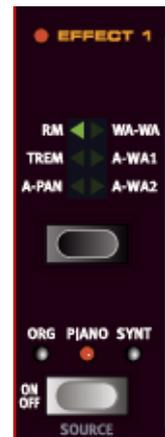
Wah-Wah modulation and you'll understand. Basically, the Wah-Wah modulation is a lowpass type of filter that can be swept across the frequency range. During the sweep, the filter's characteristics also changes. The Wah effect is mono in/out.
