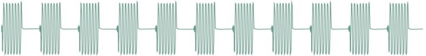
You know the trick: one oscillator playing a low-frequency square wave and another oscillator a higher-frequency sine wave, the first one resetting the phase of the second... and the two of them sent into a ring-modulator! Now roll this into one single sound generator, the parameter of which controls the frequency ratio of the two oscillators: we call it zsync... The resulting sound is close to a Jew's harp or [Morsing](#) - band-passey and formantey.
