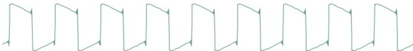
The parameter controls the pulse-width. This waveform is perfect for simulating a clarinet, for basses, “hollow” sounds or Depeche Mode-like leads. Note that this is not intended to be a perfect, drawn with a ruler, square wave. It contains a bit of high-pass filtering to make it sound more Juno-y. This waveform is band-limited and only a limited amount aliasing will be heard when playing high-pitched notes.
