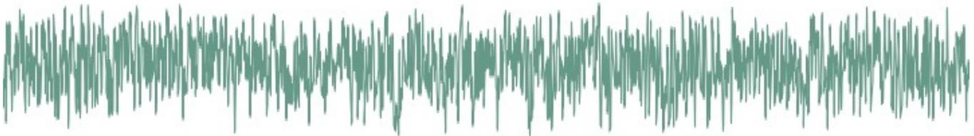
The parameter controls the frequency of a simple 1-pole low-pass/high-pass filter in which is sent white noise. From 0 to 63, high-frequency content is progressively added. From 63 to 127, low-frequency content is progressively removed. Perfect as a raw material for percussions or sound effects.
