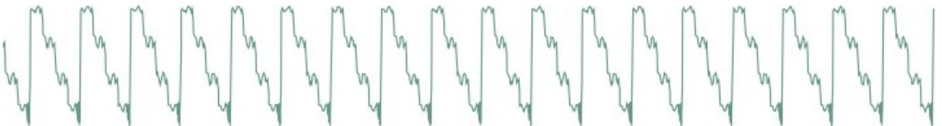
A palette of 8-bits sounding waveforms obtained by applying bitwise operations to a basic sawtooth wave (something now known as “biscuiting”).
