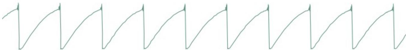
This waveform is perfect for basses and brass sounds. The parameter controls the waveshaping - when its value is increased, an increasingly large section of the waveform is shifted up. Note that this is not intended to be a perfect, drawn with a ruler, sawtooth. It contains a bit of high-pass filtering to make it sound more Juno-y. This waveform is band-limited. Thus, only a limited amount of aliasing artifacts will be heard when playing high-pitched notes.
