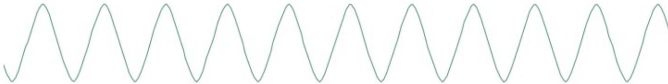
A pure waveform, which serves as a good basis for flute or soundchip-like leads. The parameter controls some kind of waveshaping, clipping the bottom of the waveform. This waveform is band-limited and will still sound fine above C5.
