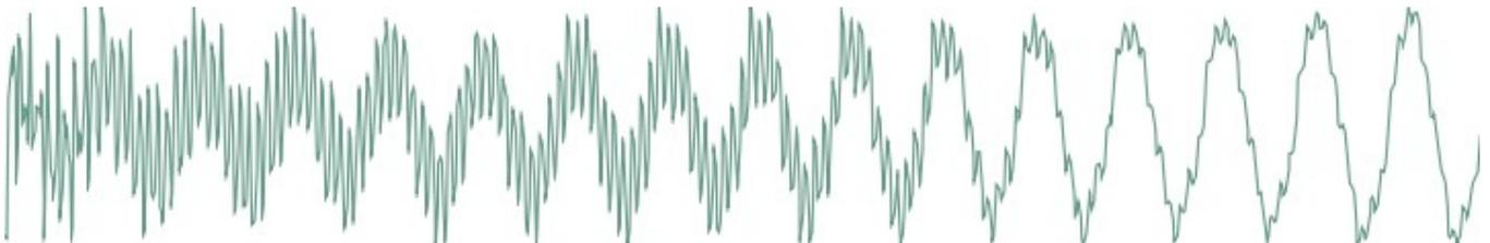
This wavetable has two peculiarities: it is smaller than the other ones (8 single cycle waveforms, each of them being 129 samples long), and it resides in RAM instead of residing in flash ROM. By default, it is loaded with the same content as **digitl**, but its content can be altered by [SysEx messages](#). You can find [here](#) some examples of MIDI files containing user wavetables.
