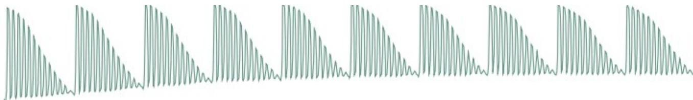
This waveform uses phase distortion to recreate a sawtooth sent through a low-pass filter with high resonance. The parameter controls the resonance frequency. Useful for doubly-filtered sounds, formants, or anything where its synthetic, cheesy, feel will shine.
