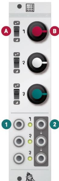
Each of the 3 channels of Shades can act as an attenuator or attenuverter.
