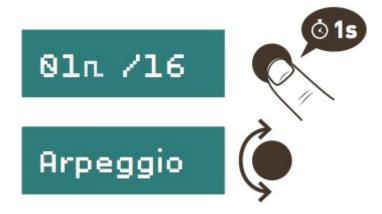
Each "feature" of the MIDIpal can be seen as an independent "app". Only one app can be running at a time - that is to say, you cannot run an arpeggiator, a drum sequencer and a MIDI monitor on the same unit! To select the app to use, keep the encoder pressed. The name of the current app is shown on the screen.
