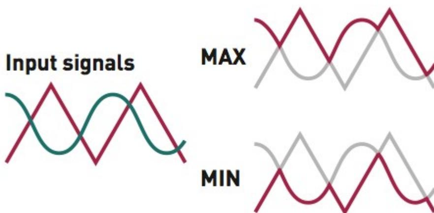
Similarly, the analog **AND** circuit extracts the minimum of the two inputs (the troughs in the graph of the two input signals).
