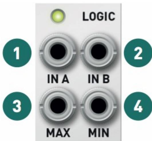
**1, 2.** Signal inputs, normalized to 0V.
