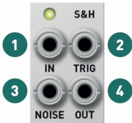
**1.** Signal input, normalized to the white noise generator.
