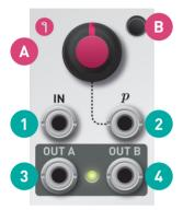
Upon receiving a trigger on its **IN input (1)**, the module tosses a virtual coin: if the outcome is heads, the trigger is sent to **output A (3)**; if the outcome is tails, the trigger is sent to **output B (4)**.
