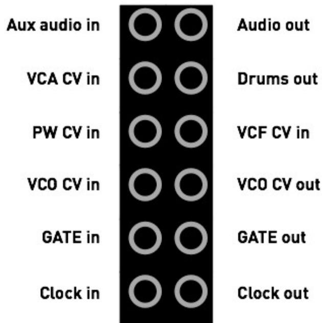
**Aux Audio in** is an additional input for external signal processing. It is activated by setting the **Sub** switch to the **DCO** position, and can be attenuated by the **Sub level** control. The input impedance is 100kΩ.
