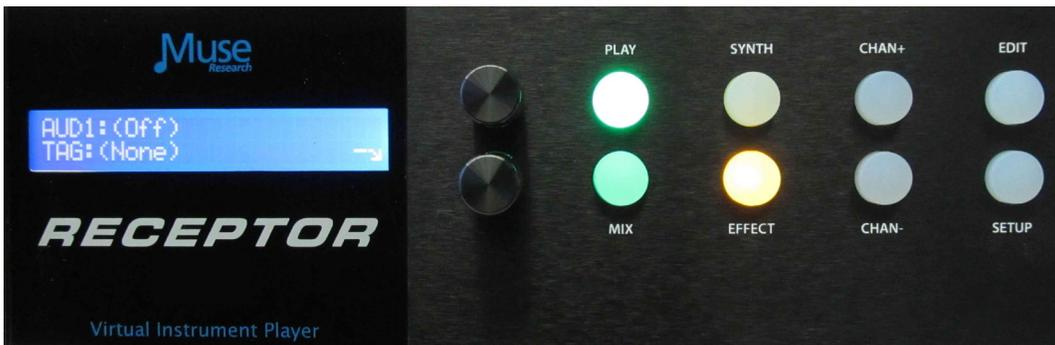
3. RECEPTOR defaults to the Stereo Line Inputs on the first channel you open up and the Mic/Gtr input on the front panel for the next channel you open up. To change the input assignment for a particular channel, simply press the SETUP button and you can re-assign the inputs to whatever input you desire. Selecting the same input across multiple channels will process the input in parallel, creating dramatic effects.
