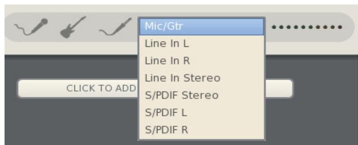
*Note: if you use the S/PDIF input, you MUST choose S/PDIF external clock option from the "Audio..." menu in the SETUP tab. Failure to do so will result in audio clicks and pops caused by errors in the data stream. By definition, digital audio inputs must have a corresponding clock source to keep the audio properly synchronized and free from data dropouts.*
