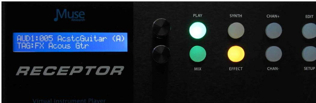
4. Bring up the gain adjacent to the front panel input, and verify that the input is not clipping when playing at your loudest level - the LED level indicator should never be red.
