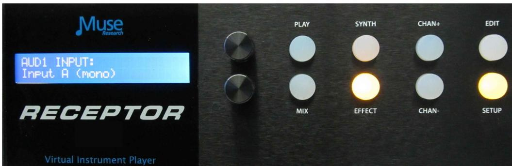
3. Turn the gain control to minimum on the front panel input and plug in your acoustic guitar. Turn the bottom encoder to select "TAG FX Acous Gtr" and then turn the top knob to select the preset "007 AcstcGuitarChannel". Press the encoder button to load the patch. Of course if there is a different preset you'd like to use on the guitar, feel free to select it now.
