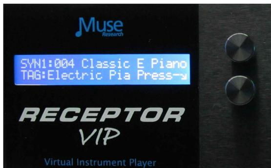
3. Now we'll layer that with another sound—say a pad synthesizer. To do this, we press the CHANNEL + button, and then the bottom encoder switch to add a new channel to what we already have loaded.
