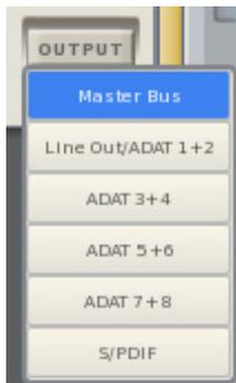
Just like a synth channel, you can alter the default routing of the output of any of the audio input channels by clicking on the OUTPUT button on the lower right hand corner of an audio channel. When you click on the OUTPUT button, you can select which outputs you want the audio channel to send to, including multiple outputs .
