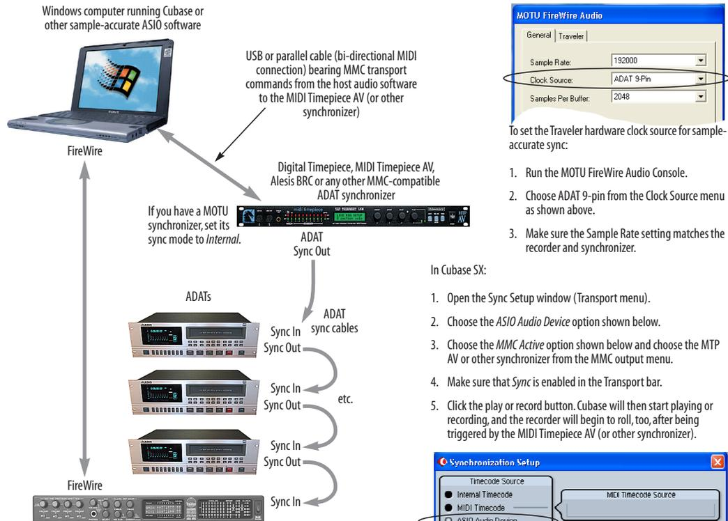
Figure 4-14: Connections for sample-accurate ADAT sync.
