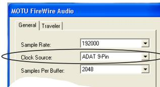
To set the Traveler hardware clock source for sample-accurate sync:
