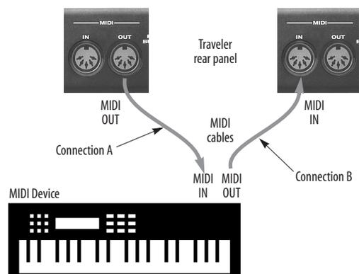
Figure 4-3: Connecting a MIDI device to the Traveler.
