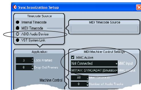
Figure 7-6: Setting up sample-accurate sync via ASIO 2.
