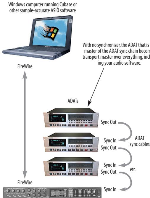
Figure 4-14: Sample-accurate sync without an ADAT synchronizer.
