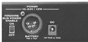
Figure 4-5: The Traveler's battery and power supply options.
