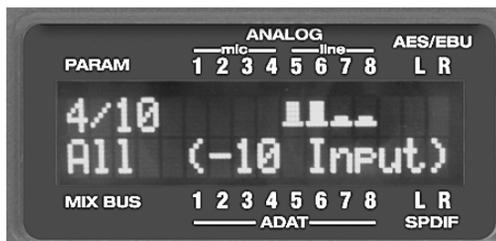
Figure 4-2: Setting the reference level for the four TRS analog inputs.
