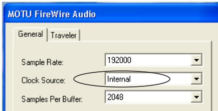
Figure 4-9: You can run the Traveler under its own internal clock when it has no digital audio connections and you are not synchronizing the Traveler system to an external time reference such as SMPTE.
