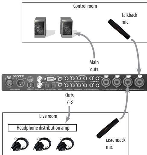
Figure 10-2: Typical hardware setup for Talkback and Listenback.
