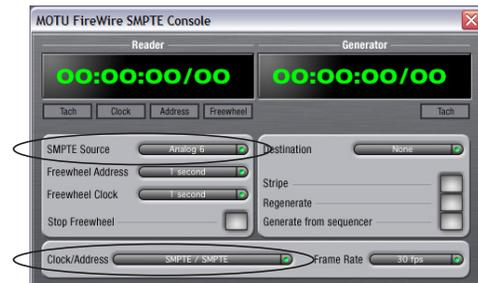
Launch the FireWire SMPTE Console and specify the *SMPTE Source*, which is the input receiving the SMPTE time code. Also, confirm that the *Clock Source/Address* is *SMPTE/SMPTE*. For details about the other settings, see chapter 11, "FireWire SMPTE Console" (page 79).
