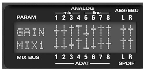
Figure 6-4: In mixer mode, the LCD displays the mix settings for the mix bus currently being displayed in the LCD.
