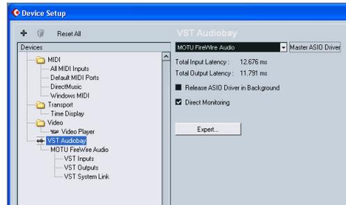
Figure 7-2: Activating the Traveler FireWire ASIO driver in Nuendo and Cubase.
