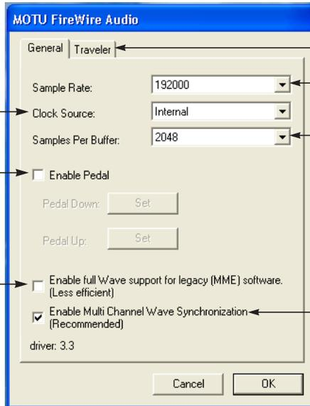
Click the tabs to access general MOTU FireWire interface settings or settings specific to the Traveler (or other connected interface.)
