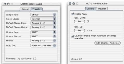
Figure 7-1: Choose Setup menu> Configure Audio System> Configure Hardware Driver to open the dialog shown above and access the Traveler Core Audio driver. To access the rest of the Traveler settings, open the MOTU FireWire Audio Console.
