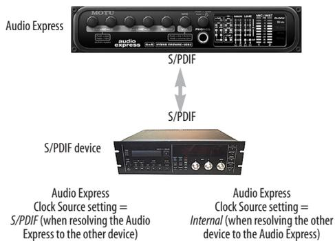
Figure 4-5: The setup for synchronizing a S/PDIF device with the Audio Express. Sync is achieved via the digital I/O connection itself. In this case, you have to choose S/PDIF as the Audio Express's clock source when resolving it to the other device.
