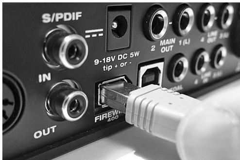
Figure 4-1: Connecting the Audio Express to the computer via FireWire.
