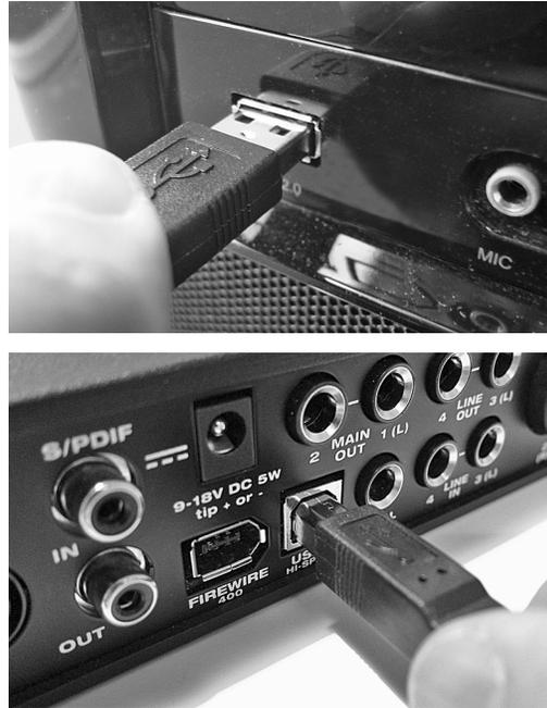
Figure 4-2: Connecting the Audio Express to the computer via USB.
