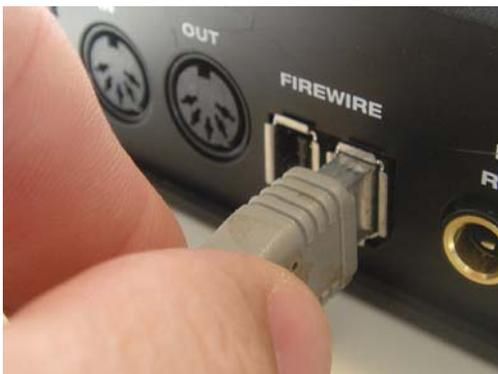
Figure 4-1: Connecting the 8pre to the computer.
