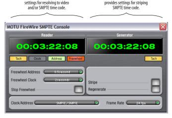
Figure 11-1: SMPTE Console gives you access to your 828mkll's on-board SMPTE time code synchronization features.
