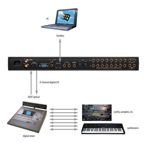
Figure 4-6: Using the 828mkll with a digital mixer.
