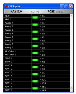
Figure 7-3: Activating 828mkll inputs in Cubase VST.
