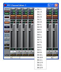
Figure 7-5: To assign an 828mkll input to a Cubase VST audio channel: control-click the input button at the top of the channel strip. For Nuendo or Cubase SX, consult your documentation.
