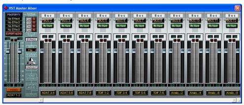
In Nuendo or Cubase SX, access the 828mkll outputs via the busses in the VST Outputs window.
