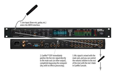
Figure 9-2: This diagram shows the signal flow when using CueMix $^{\text{TM}}$ DSP no-latency monitoring. Notice that this method does not allow you to process the live input with plug-ins in your audio software while it is being monitored. You can, however, add effects later — after recording the live input as a disk track. CueMix $^{\text{TM}}$ DSP lets you hear what you are recording with no delay and no computer-based effects.
