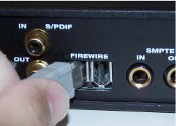
Figure 4-1: Connecting the 828mkll to the computer.
