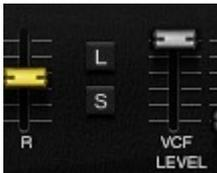
You will find group presets save and load for synthline1, synthline2, performance section and equalizer. "L" means load. "S" means save.
