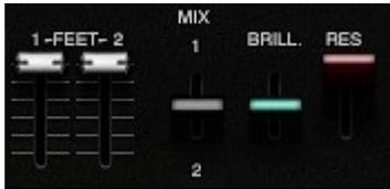
Feet: Octave settings for the oscillator pitch. Tuned in fifths and octaves.
