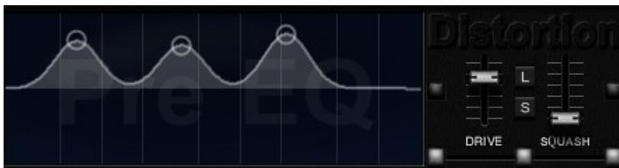
3 band EQ pre and 3 band EQ post. At the bottom there are off/on switches for eq and overdrive. When overdrive is "off" you can use the both EQs as a big 6 band Equalizer. Volume compensated overdrive. You can adjust EQ with GUI or old-style knobs. Midi-learn (and unlearn) for all bands. It is a Fully Parametric EQ; Frequency, Gain and Width(Q) controls - All can be automated or set to MidiCC/NRPN. Midi-learn implemented in the old-style knobs.
