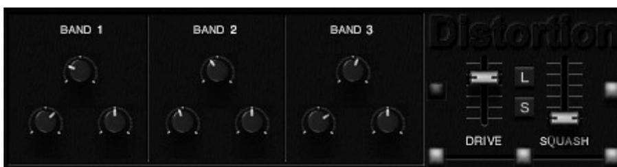
Drive: This sets the distortion Sound. It sets the amount of signal Gain or boost before it enters the distortion and equates to 'Amount of distortion'.
