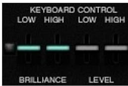
This section makes it possible to alter the instruments response for the upper and lower keys on the keyboard. Middle slider position is default. The curve is exp as you move from the middle part of the keyboard. It is often used to increase the level of the lower keys, since they may feel weak because of the instruments built-in aggressive keyboard filter scaling. For more information: Read the YAMAHA CS80 manuals.
