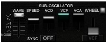
The sub-oscillator is the instrument`s LFO.
