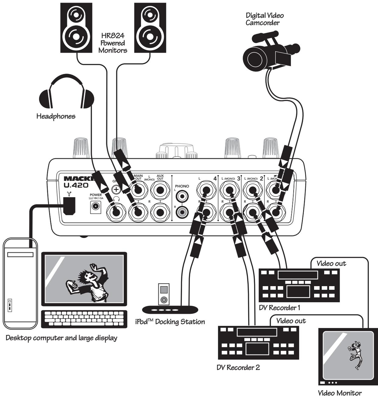
*This diagram shows a DV camcorder audio connected to channel 1, DVR decks connected to channels 2 and 3, and an iPod docking station connected to channel 4.*
