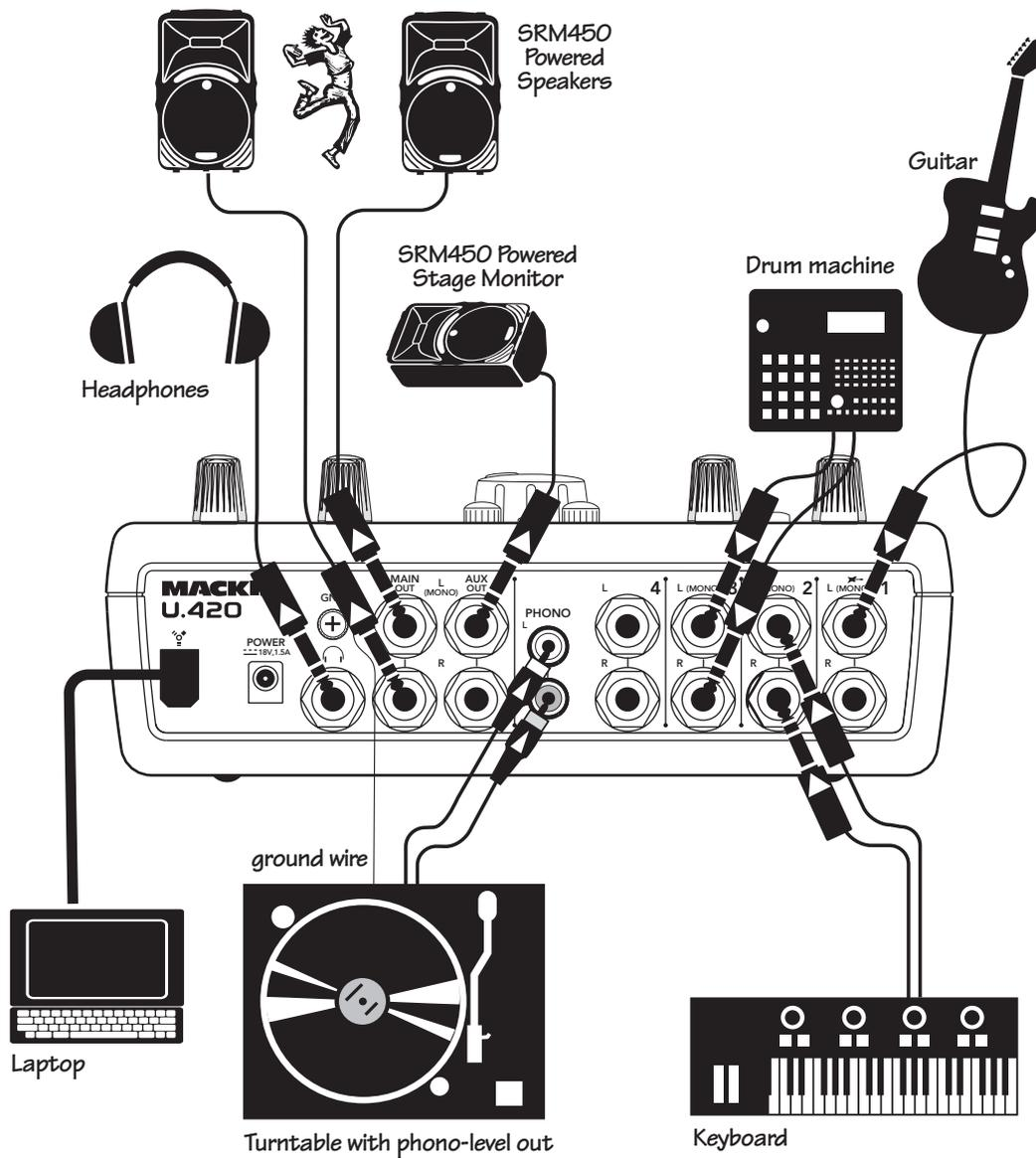
This diagram shows a guitar connected to channel 1, plus a stereo synth and drum machine connected to channels 2 & 3. A turntable is connected to the phono inputs on channel 4. Use the left aux send to connect to a Mackie SRM450 for stage monitoring. The U.420 will automatically sum the stereo signal to mono if you use the left aux output only.
