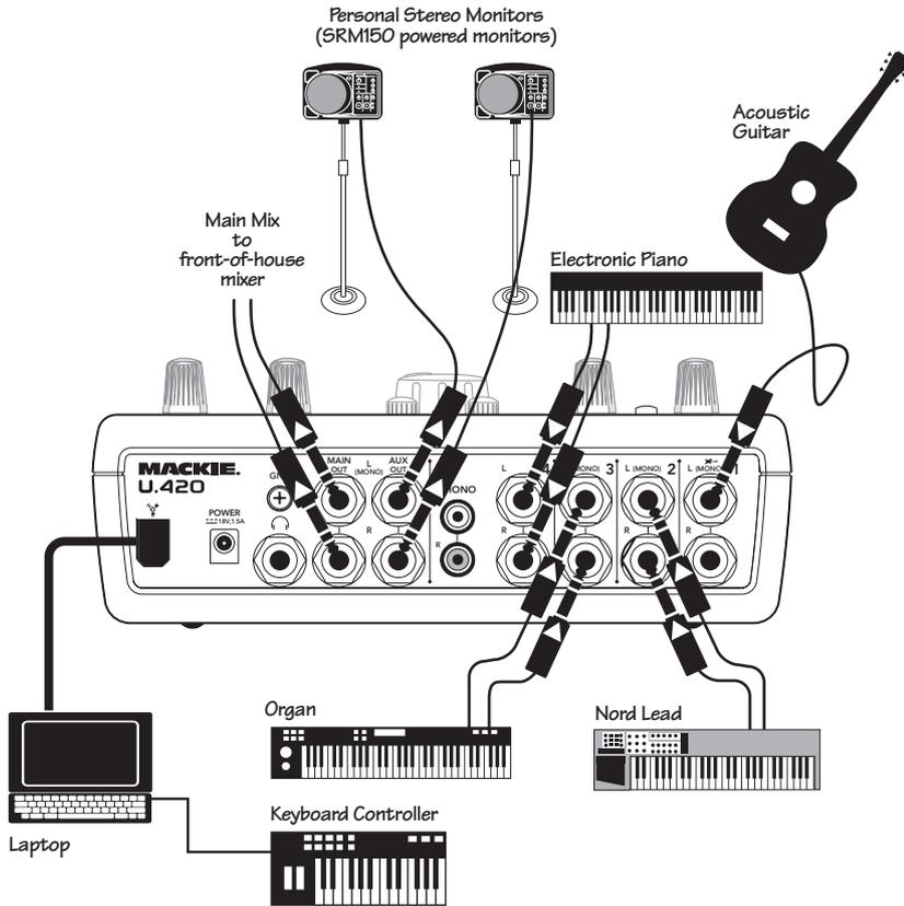
This diagram shows an acoustic guitar connected to channel 1, plus a stereo performance synth like a Nord Lead on channel 2, a good organ like a Korg CX-3 on channel 3, and an electronic piano on channel 4 (with a dab of channel #5 behind each ear for good measure).
