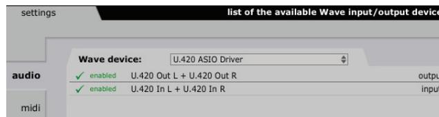
3. Play a source into the U.420 and verify that your software is receiving the signals correctly.
