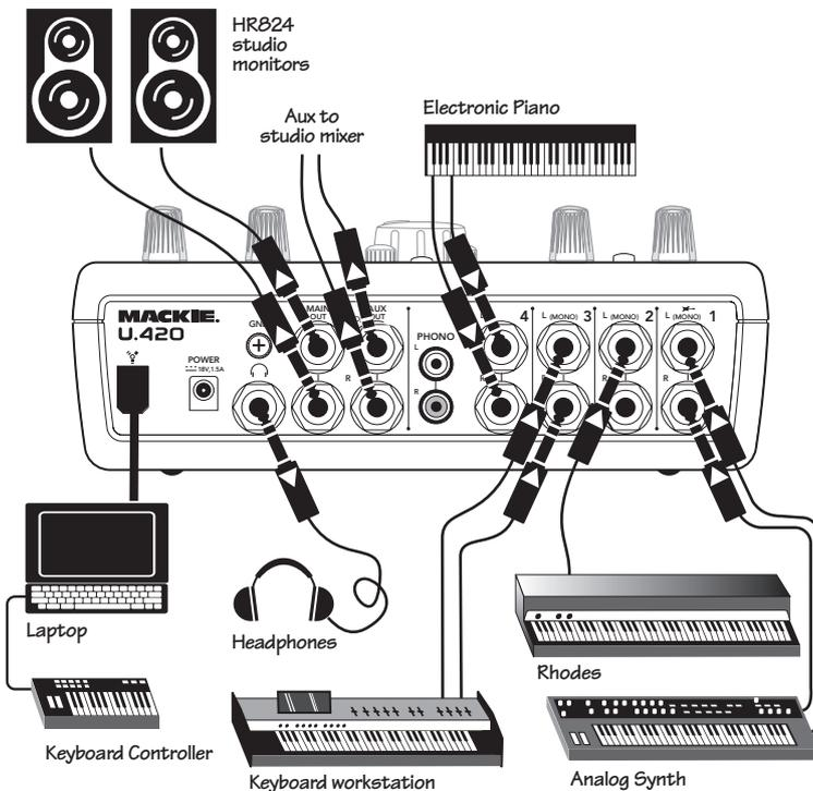
This diagram shows a stereo keyboard workstation, a groovy analog synth, an electronic piano, and an electric organ connected to channels 1-4.
