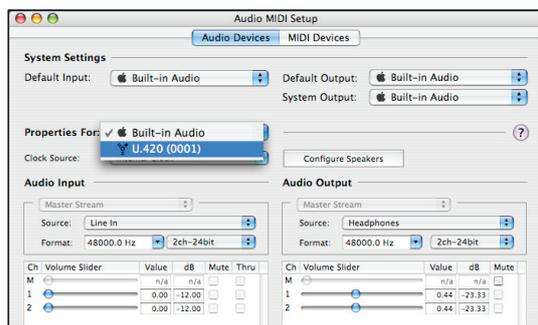
4. Here you can see the settings for the U.420. You can also choose the U.420 as your default input or output, as well as designate it to be used for the system sound output.
