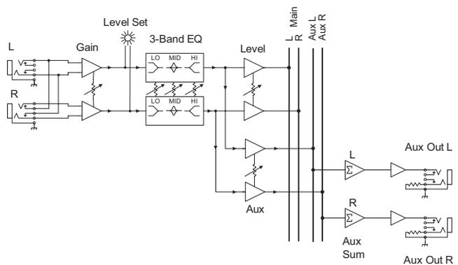
The channel signals go through the preamplifier and into the EQ. The level control [17] allows you to adjust how much of the channel appears on the main mix bus. The aux control [16] allows you to adjust how much of each channel appears on the aux bus.
