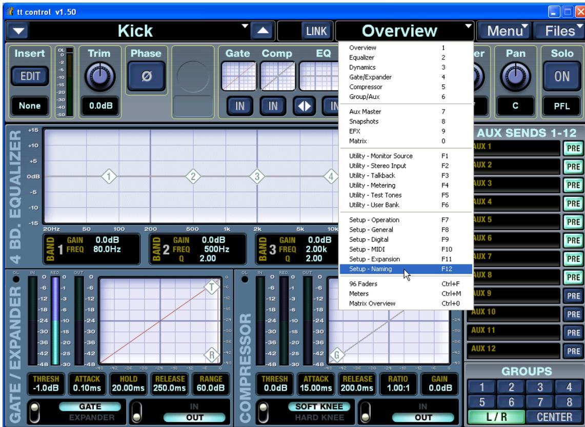
Like the Touchscreen, a two-column list shows the channel default names on the left and any custom names on the right. Click the RENAME button and enter the new name in the “Set Channel Name” popup. Channel names can be up to 6 characters long. You can use the up/down arrow keys on your keyboard to scroll to the previous/next channel for renaming. Press Enter or click OK when finished renaming.
