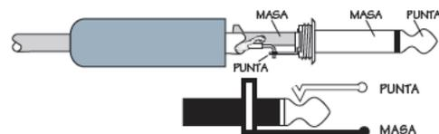
Figura C: conector TS
