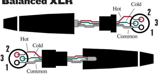
Standard XLR microphone connector to be used with mic-level.
