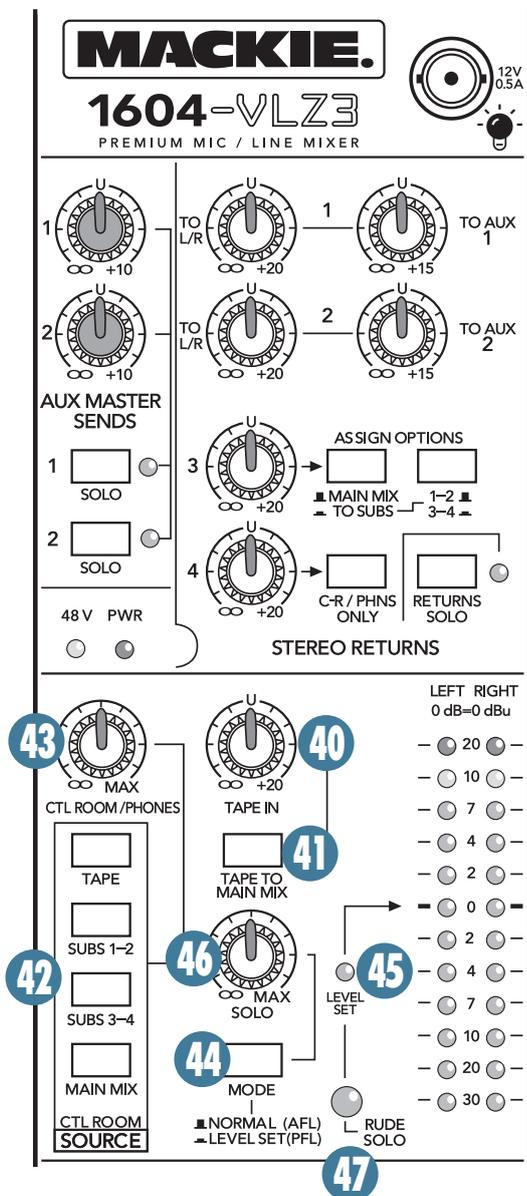
Engaging a SOLO switch will cause this dramatic turn of events: Any existing SOURCE matrix selections will be replaced by the SOLO signals, appearing in the control room, headphones and meter display. The audible solo levels are controlled by the SOLO [46] level knob. The SOLO levels appearing on the meter display are not controlled by anything — you wouldn't want that. You want to see the actual channel level on the display, regardless of how loud you're listening.
