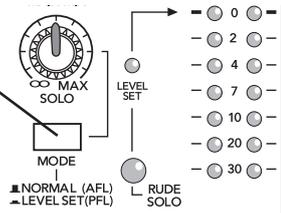
**VERY IMPORTANT** LEVEL SET (PFL) taps the channel signal before the fader. If you have a channel’s fader set way below “U” (unity gain), SOLO won’t know that and will send a unity gain signal to the control room, headphones, and meter display. That may result in a startling level boost at these outputs, depending on the position of the SOLO [46] level knob.
