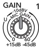
Through the 1/4" input (LINE), there is 15 dB of attenuation fully down and 45 dB of gain fully up, with a "U" (unity gain) mark at 10:00.
