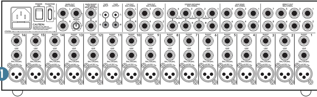
At the risk of stating the obvious, this is where you plug everything in: microphones, line-level instruments and effects, headphones, and the ultimate destination for your sound: a tape recorder, PA system, etc. A few of the features described in this section are on top of the mixer, but most are out back on this “pod.”
