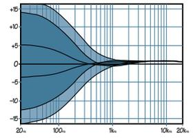
Used in conjunction with the LOW CUT [33] switch, you can boost the LOW EQ without injecting a ton of subsonic debris into the mix. We recommend using the LOW CUT feature on all channels, except low frequency signals, like kick drums and bass guitars.
