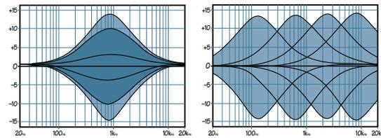
Most of the root and lower harmonics that define a sound are located in the 100 Hz–8 kHz frequency range, and you can create drastic changes with these two knobs. Many engineers use MID EQ to cut midrange frequencies, not boost them. One popular trick is to set the MID fully up, turn the frequency knob until you find a point where it sounds just terrible, then back the MID down into the cut range, causing those terrible frequencies to disappear. Sounds silly, but it works. Sometimes.
