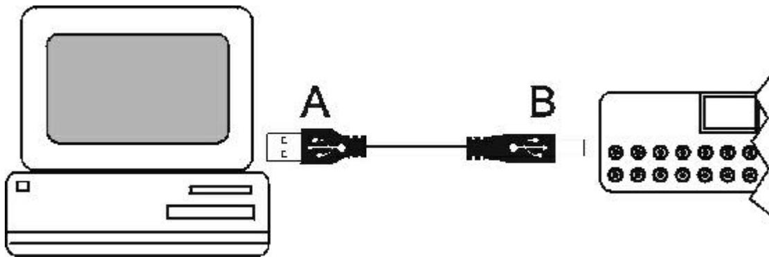
This cable provides the UC16 with its power. Switch the UC16 on and the red LED display will light up.
