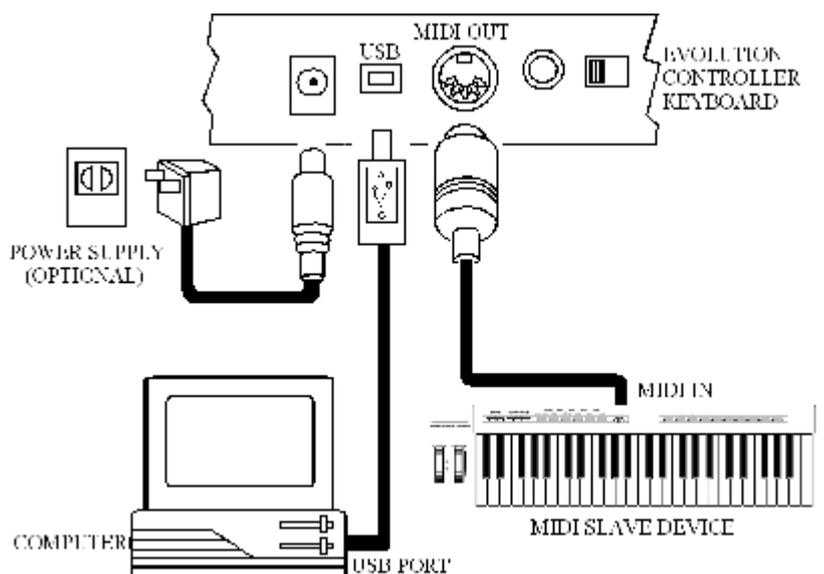
Data can be sent to the MIDI slave device from the computer by selecting 'MIDI out from USB' on the UC16. To do this press the Control Assign and Control Select buttons simultaneously.
