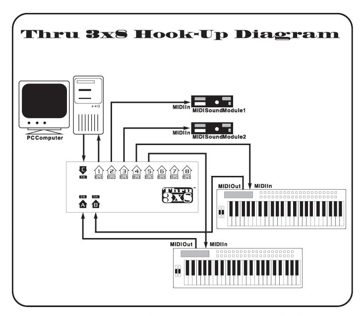
The Thru 3x8 uses a 9 volt, center pin positive wall adaptor for power (300 milliamp minimum). To power the unit up make sure that a suitable adaptor is plugged into the power jack on the back of the unit and also plugged into the wall. Next, depress the power switch on the front left panel. If everything is done correctly, the power LED over the power switch will light.
