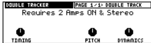
Unlike the other buttons in the Function row, The Double Tracker works as an Effect On/Off button. Specifically: If the Double Tracker button is lit, the effect is active. To edit Double Tracker parameters, the Edit button must be pressed. If Double Tracker was not the last effect accessed, the Double Tracker button must also be pressed.
