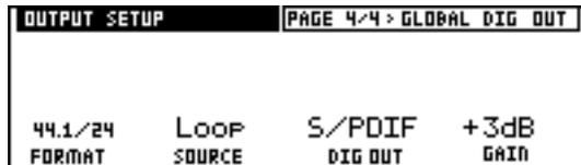
Page 4 of Output Setup is where you will make these settings. The first parameter is FORMAT. This is where you set the bit depth and sample rate coming from the Vetta. Use the soft knob under FORMAT to change this parameter. You have the choice of
