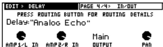
Depending on the Routing Configuration that you've chosen (see page 4•18), AMP1/L IN and AMP2/R IN determine either (1) how much of each amp feeds the delay or (2) how much of the left and right outputs of the previous effect feed the delay. The OUTPUT knob determines whether the delay will be sent to the Main outs or the Wide outs, if you've got Wide Mode turned on (page 4•34). MIX determines how much of the delayed signal is mixed in relative to the rest of your signal.
