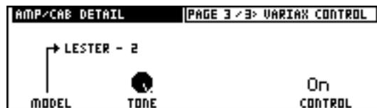
The MODEL parameter is where you choose which Variax instrument model you wish to recall with the Vetta channel. The first choice you have for the MODEL parameter is “None.” With this setting the Vetta will not change your Variax’s MODEL or TONE when this Vetta channel is recalled. The setting is also controllable directly from the Variax’s Model and Pickup Selector switches.
