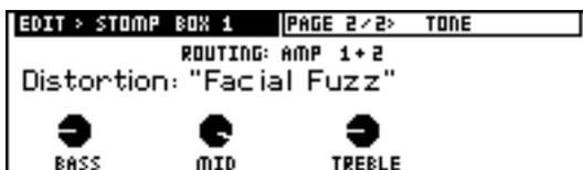
Here you've got tone controls (BASS, MID, and TREBLE) for each distortion. As you'll notice in the descriptions that accompany the list of models below, some of these controls model the behavior of controls from the original box that we studied to create our models, and some add new functionality.
