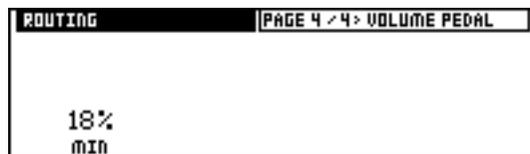
This minimum value determines how much volume you'll hear when the volume pedal is at the heel position. The heel position normally turns the volume off (a setting of 0% for the MIN value), but you may find it preferable to set it so the heel position is not all the way off. This comes in handy, for instance, when you want to
