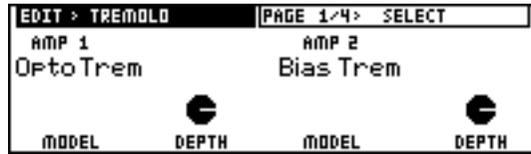
Page 1 lets you pick the tremolo MODEL to be used with each amp, and set the DEPTH of the tremolo—how much the tremolo brings the volume down with each pulse. At 100% Depth, the volume goes all the way off with each pulse. 0% Depth is off, so you can easily have tremolo on one amp and not on the other.
