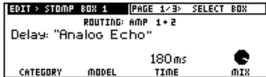
In this example, the display says “ROUTING: AMP 1 + 2”, meaning this stompbox is routed to feed both amps (see page 4•18 for Routing details). Since the stompbox is feeding both amps, this means that whether you have Amp 1 or Amp 2 turned off, you’ll hear the stompbox. If you *did* have a stompbox routed to Amp 1 only, and Amp 1 was off, you would, of course, not hear the stompbox even if you turned the stompbox on. Just like *real* amps and stompboxes, right?
