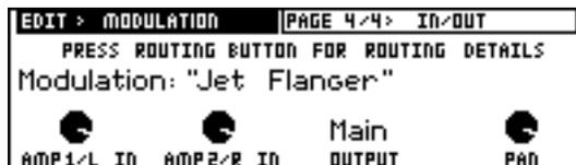
These controls all work just like their cousins on the Pitch Shift's page. In fact, all the Routable Post Effects share this same last page for adjusting the inputs and outputs for the effect.
