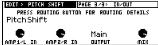
Depending on the Routing that you've chosen (see page 4•11), AMP1/L IN and AMP2/R IN determine either (1) how much of each amp feeds the pitch shift or (2) how much of the left and right outputs of the previous effect feed the pitch shift. The OUTPUT knob determines whether the pitch shift will be sent to the Main outs or the Wide outs, if Wide Mode is on (page 4•34). MIX determines (surprise!) how much of the pitch shifted signal is mixed in relative to the rest of your signal.
