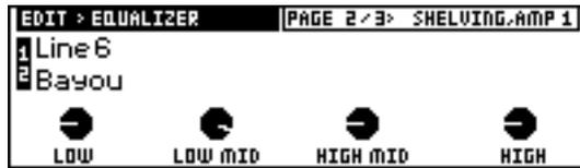
Each band has  $\pm 12\text{dB}$  of range available. Set a knob to 12 o'clock for no boost or cut for that band. The center frequencies for the 4 bands are 80 Hz, 200 Hz, 800 Hz, and 3 kHz.
