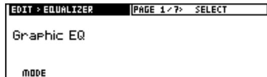
Twist the knob below MODE to select either the Graphic EQ or the 4-Band EQ. Whichever mode you choose, you’ve got independent processing for each of the two amp models.
