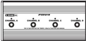
The FBV4 has 4 switches labeled A, B, C and D. These switches allow you direct access to any of the four channels in the current bank. An LED will light showing you the currently selected channel. Repeatedly pressing the currently selected channel switch will result in changing the tap tempo time in the Vetta.
