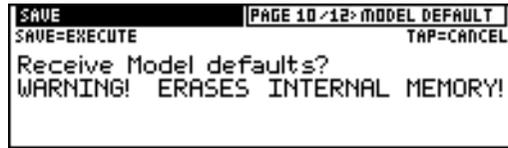
Now you have to clear Vetta's current Model Default memory so it has the space required to receive the MIDI dump. Press the Save button while this page is showing, and you'll see the message "Erasing model defaults." When it's finished, another message says "Ready to receive model defaults." You can then start transmitting the MIDI dump from your MIDI setup.
