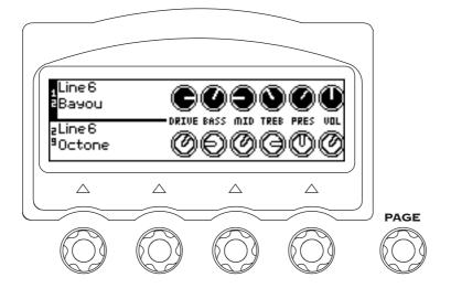
The normal display state, called the Amps At A Glance Page, shows which amp models you've got going, and how their Tone Controls are set; this is detailed in the Basic Operations chapter. In this state, the knobs below the display don't function.
