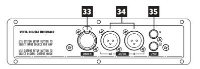
**33. Variax RJ-45 Digital Input:** This allows for digital connection from the Variax modeling guitar to the Vetta. Vetta will supply power to the Variax from this connection. Variax settings can be stored and recalled within Vetta channels when this input is used. Connection can be made with the included locking Variax cable or with any standard CAT 5 Ethernet computer cable.
