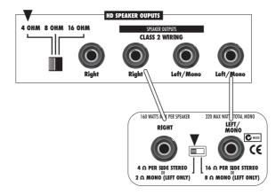
Hooking up your Vetta HD in side by side stereo with two 4x12s
