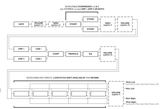
MIXED SERIES, PARALLEL AND CHAIN ROUTING AVAILABLE. ALL PARALLEL ROUTING SHOWN HERE.
