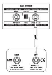
With this wiring, you can only use Vetta's Split mode. You can, of course, run an 8 ohm or greater cabinet wired like this, but we can't guarantee that you'll get the best balance of level between the amp and extension cab because Vetta's left and right power amps will be loaded unevenly. You'll run into the same uneven loading problem if you try and run an 8 ohm cabinet wired like this in Normal mode.
