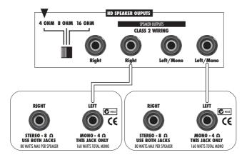
Hooking up your Vetta HD in stacked stereo with two 2x12s
