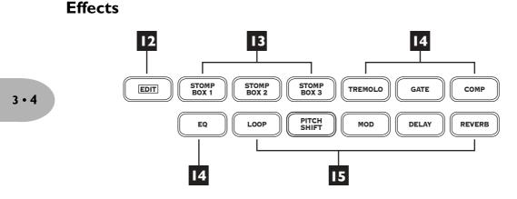
Here's where you control and setup all your effects. The basic brain dead mode of operation is light on, effect on. Light off, effect off. All the effects work at the same time (with the exception of Pitch Shift and Modulation), to achieve any level of moderation or excess you desire. Press the Edit button to dive deep into the details of any effect and tweak it to make it your own.
