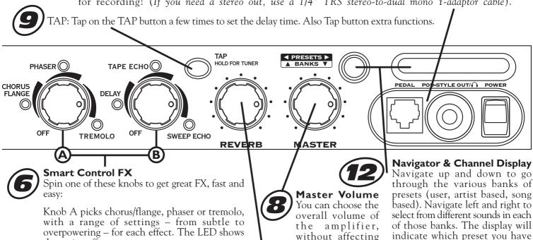
Knob B picks delay, tape echo or sweep echo, with a range of mix settings from low to high. The LED shows the active effect and flashes the delay time. Tap the TAP button to change the delay time.
