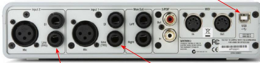
From your Line 6 device’s **Right Analog Out** (or “**Out 2**”), connect to the Mbox 2 **Input 2 - Line input**
