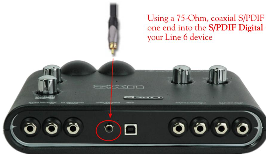
Using a 75-Ohm, coaxial S/PDIF cable, plug one end into the **S/PDIF Digital Out** of your Line 6 device
