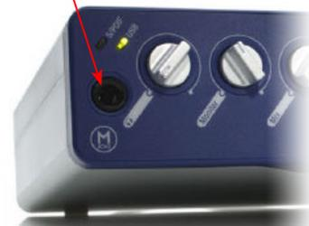
From the Mbox **Mon Out** jacks, connect to the Left and Right inputs for your powered speakers or monitoring system
