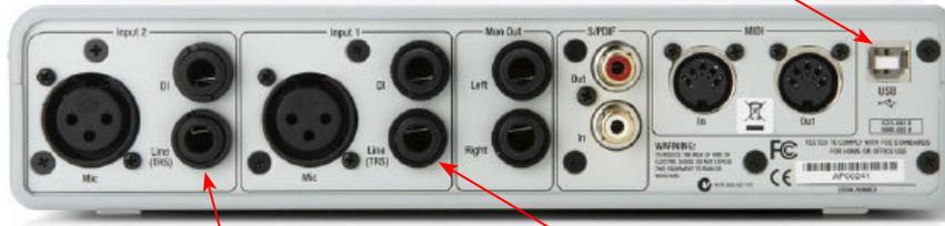
From your Line 6 device’s Right Analog Out (or “Out 2”), connect to the Mbox 2 Input 2 - Line input
