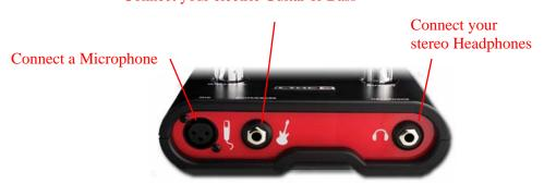
**Mic** - To input a signal from a microphone, connect it here using and XLR cable. This inputs the microphone signal into GearBox where you can choose your tone, and then route the processed signal both to your audio software and out the TonePort outputs.
