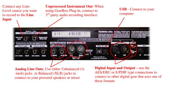
**Line Input** - if you want to record the signal from a line level source, such as a keyboard, your receiver, the line out from a mixing console, etc..., connect it to this input using a 1/4-inch TS audio cable.
