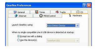
If your Line 6 hardware is connected to your computer and it's not available from the "Launch GearBox using:" menu there, there is a USB connection error. It is specifically recommended to always connect your Line 6 device directly to your computer's USB port, and **not** into a USB hub. USB hubs can sometimes cause communication errors with USB audio devices.
