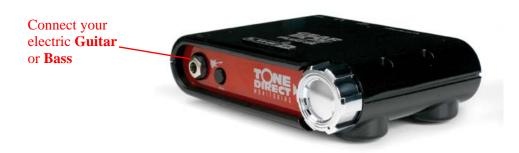
**Guitar/Bass** - To input your electric guitar or bass, plug it in here using a standard 1/4-inch TS instrument cable. This input also features a **Pad switch**; engage this switch when using a guitar/bass with high-output or active pickups, to avoid overdriving the input.
