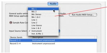
When GearBox is not in use, the Input Source Select menu is available. As shown here, TonePort devices offer several input Sources to choose from. The selected Source is what gets routed to the Device Sends.
