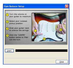
The **Hum Reducer** reduces the noise that your guitar (or bass guitar) puts out\*, including noise that is caused by electrical interference from your computer display and other sources that are picked up by your guitar's pickups. The Hum Reducer will not completely eliminate hum, but it is usually able to reduce it considerably. To use the Hum Reducer:
