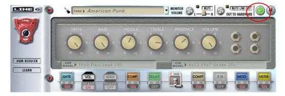
Note, for PODxt, the Bypass button functions as an Amp Bypass only, where only the amplifier processing is bypassed, and any effects that are active are still applied to the input signal by your PODxt.
