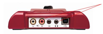
Connect a 1/8-inch stereo cord to the **Headphone Out**, or use the Stereo **RCA Line outputs** with an adapter.
