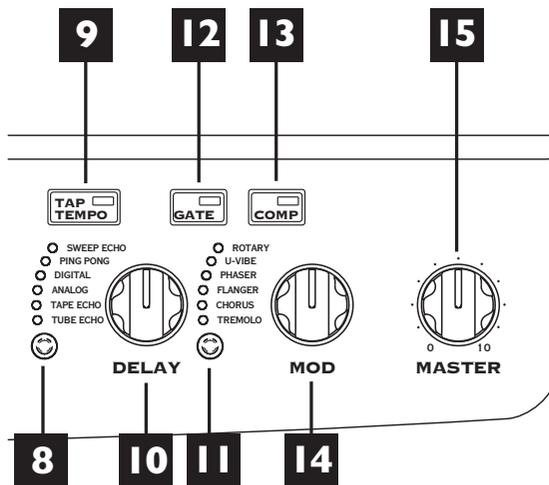
8. **Delay Select:** Press this to step through the Delay effects listed to the left of the Delay knob, or to turn off the Delay (all lights off).
