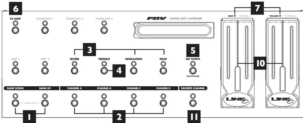
1. **Bank Up - Bank Down:** Use these two switches to choose any of the 9 Banks of Flexitone III Channel Memories. Bank 1 is the same four memories you get from the front panel **A, B, C, D Buttons** when no FBV is connected, or an FBV4 is used.
