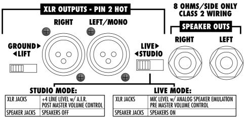
Plus/XL rear panel shown here. HD jacks and switch are at right side of rear panel
