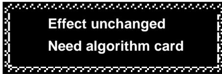
A placeholder is transmitted for any register which cannot be dumped due to the absence of an algorithm card. This placeholder contains the program name and algorithm number, but no effect parameter data. This allows an editor to identify registers which were not sent, and the algorithm card which must be loaded to complete the dump. The PCM 90 will always ignore the placeholder, and will display the following message when a placeholder is received:
