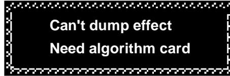
If you do not have the algorithm card loaded into the *receiving* PCM 90 when a valid SysEx for an effect created from a card algorithm is received, the following message is displayed:
