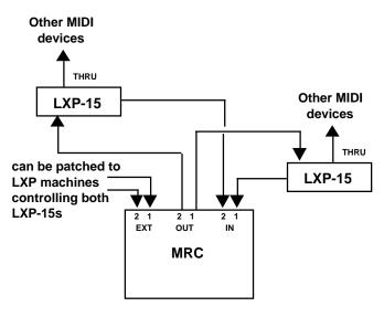
Using two-way communication you can control two LXP-15s, one for each input/output pair. If you have a high quality MIDI merger you can control multiple LXP-15s on the same input/output pair. (Each LXP-15 and its corresponding MRC machine must be assigned to a different MIDI channel.)
