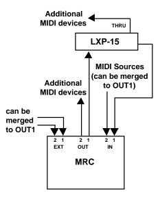
When connected for two-way communication, the merging function for the input port connected to the LXP-15 must be set to "OFF" (If it is set to "ON," communication will not be possible and the MRC will display "SYNCH TIMEOUT")
