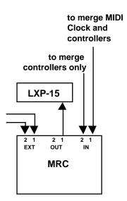
When connected for one-way communication, you can use the merging features of the MRC to route MIDI controllers from either MIDI input to the LXP-15. This is useful when you are using an LXP-15 register that uses MIDI sources for patching. Merging functions are selected on page 1 of the SYSTEMS PARAMETERS menu. The different merging options are outlined in the following table:
