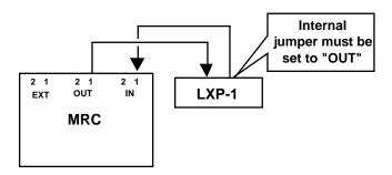
When connected for two-way communication, the merging function for the input port connect to the LXP-1 must be set to "OFF" (If it is set to "ON," communication will not be possible and the MRC will display "SYNCH TIMEOUT")
