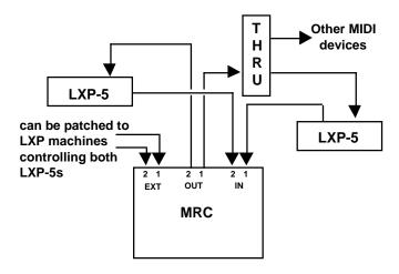
Using two-way communication you can control two LXP-5s at once, one for each input/output pair. If you have a high quality MIDI merger you can control multiple LXP-5s on the same input/output pair. (Each LXP-5 and its corresponding MRC machine must be assigned to a different MIDI channel.)
