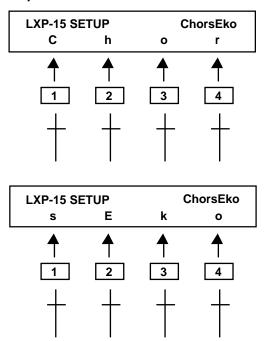
Use the sliders and switches on these two display pages to change the setup name. Each slider/switch selects one of the eight characters in the name.
