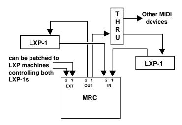
Using two-way communication you can control two LXP-1s at once, one for each input/output pair. If you have a high quality MIDI merger you can control multiple LXP-1s on the same input/output pair. (Each LXP-1 and its corresponding MRC machine must be assigned to a different MIDI channel.)
