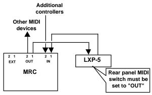
When connected for two-way communication, the merging function for the input port connected to the LXP-5 must be set to "OFF" (If it is set to "ON," communication will not be possible and the MRC will display "SYNCH TIMEOUT"
