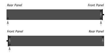
3. Remove the top cover by gently sliding it straight back, away from the front panel as shown in the figure at the top of the next page.
