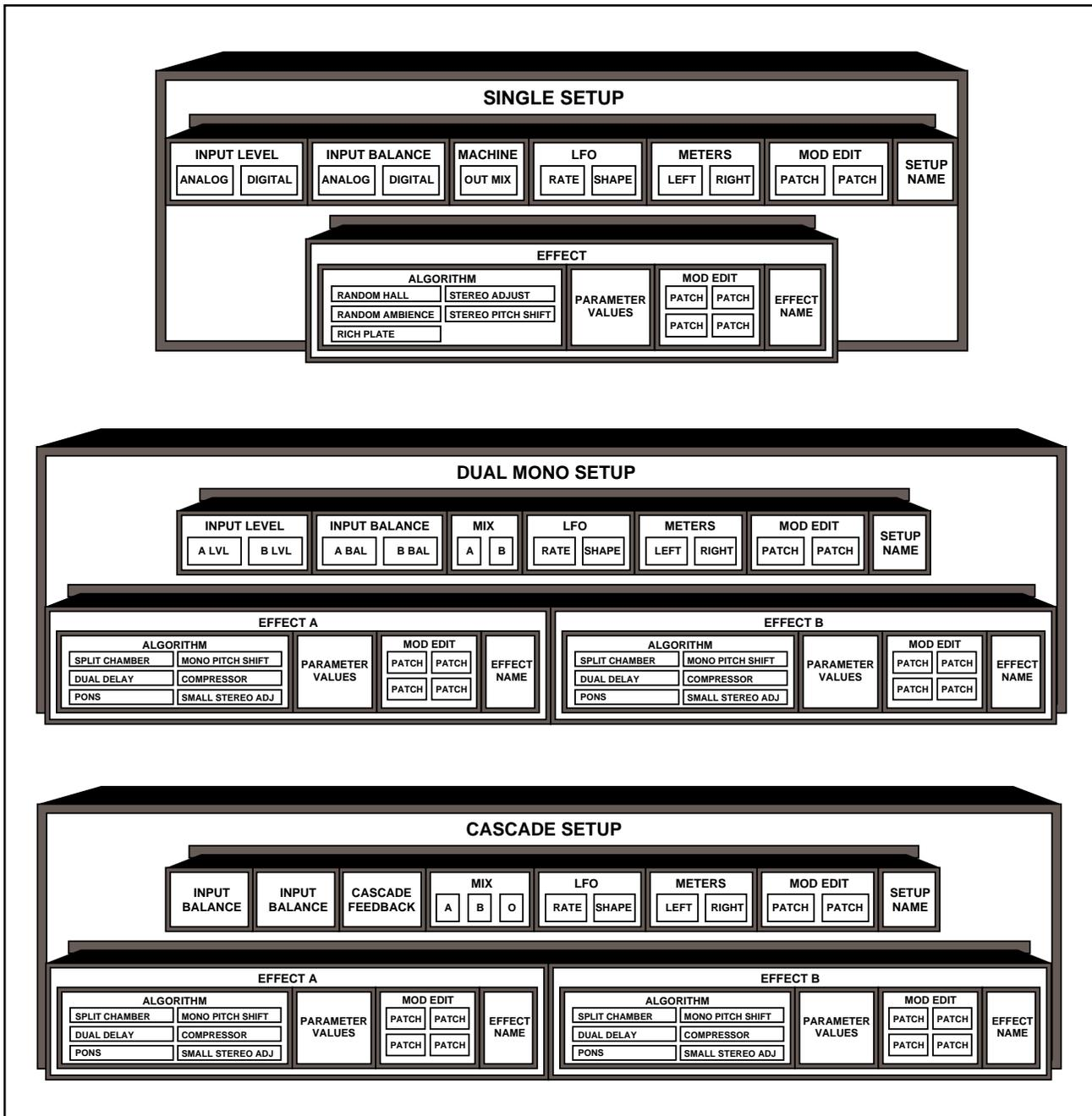
When the 300 is powered up, the SETUP SELECT button should be lit, indicating that the unit is in Setup Select mode. Turning the Soft knob will cue a new setup into the display window. Pressing ENTER will load the new Setup — and the Effect(s) associated with it.
