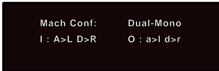
In this format, analog audio feeds the Input to the Left Processor (Machine A); digital audio feeds the Input to the Right Processor (Machine B).
