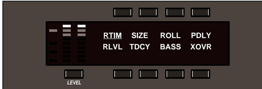
Once selected, parameters can be adjusted over their entire range with the Soft knob. The parameter and its current value will appear on the display as long as the Soft knob is being adjusted.
