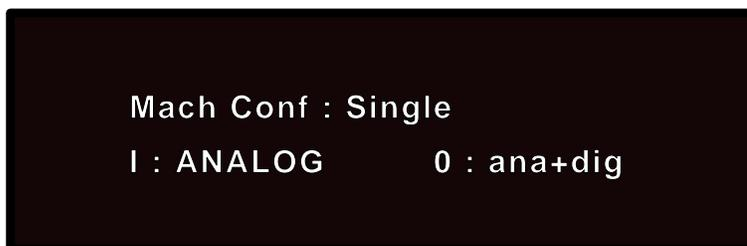
Before turning the Soft knob to change the Input type, press PAGE DOWN to display the Digital Input and Sampling Rate page. This page allows you to select different types of Analog and Digital I/O parameters.
