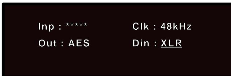
Inp: Indicates the Digital Format if properly locked. If \*\*\*\*\* appears, the 300 is not locked to an external digital sync.
