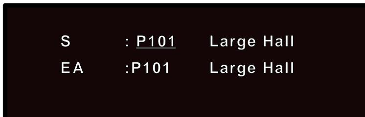
Page One allows selection of a setup. The upper line indicates "S:" (setup), a preset (P) or register (R) number, and the setup name. The upper row of buttons will step sequentially through the list of setups; turning the soft knob will scroll through the list. After finding a setup you want to load, note its number. There are two ways to load this setup:
