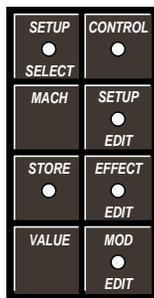
Pressing the front panel VALUE key will display all of the current parameter values for the selected page. In this example, pressing VALUE will cause the following display to appear:
