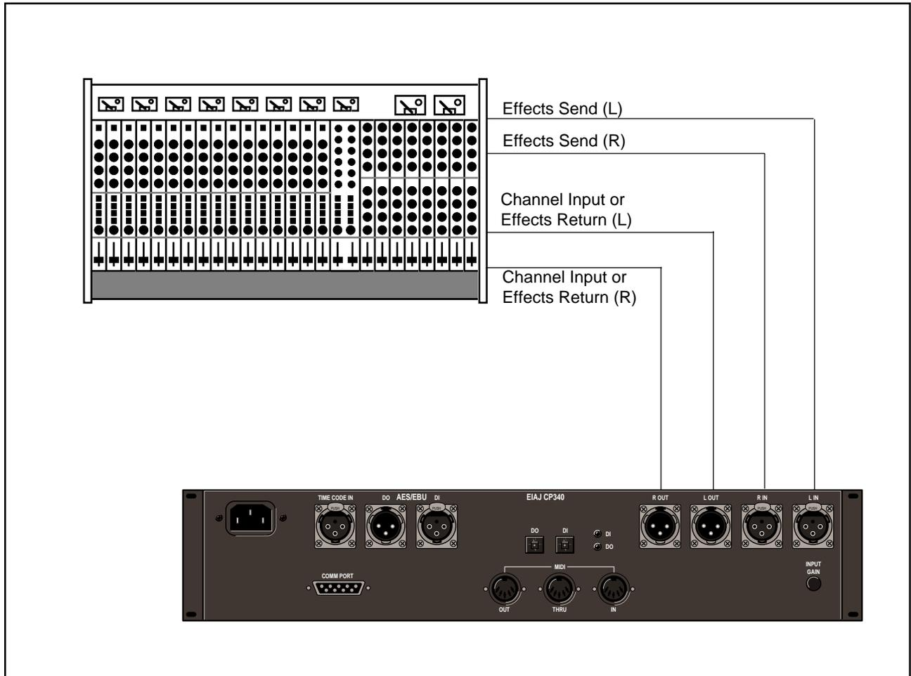
If you will be using a 300 as your primary effects unit, and your system includes a console with one or more auxiliary (effects) sends, connect the 300 as shown above. In most applications, it is preferable to connect the 300 outputs to two of the console's input channel strips, panned full left and right, rather than the effects returns. This allows the greatest flexibility in routing and equalization.
