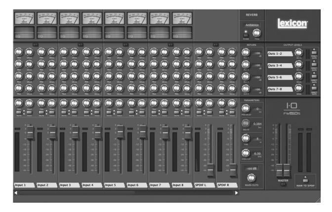
The IO FW810S includes a powerful hardware Mixer with a software control panel and built-in EQ, dynamics, and monitor reverbs. When open, the Mixer controls the IO FW810S hardware. The controls are described in more detail on the following pages, and a step-by-step example project can be found in the Tutorial at the back of this manual.
