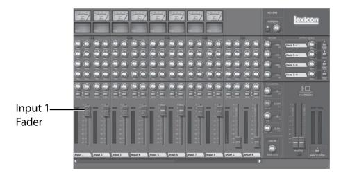
6. Play the guitar and note the meter in the Mixer's Input 1 strip; it should be moving, indicating a signal is present. If the meter isn't indicating a signal while you play the guitar, turn up the Gain 1 knob on the IO FW810S until it does. Aim for a peak signal level which does not exceed -6 dB on the meter when the guitar is strummed.
