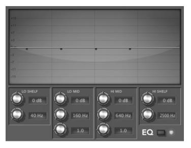
Inputs 1-8 in the Mixer feature a parametric EQ where you can cut or boost selected frequency bands. You can edit parameters with the control knobs (described below), or you can click and drag the anchor points in the EQ's display (shown above). To open or close the EQ for a specific channel, click the EQ indicator/button just below the Gain Reduction meter/button for that channel.
