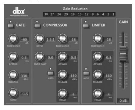
Inputs 1-8 in the Mixer feature Channel Strip Dynamics, including a gate, compressor, limiter, and a gain fader. To open the Channel Strip Dynamics, click the Gain Reduction meter/button at the top of the channel's "strip" in the Mixer.
