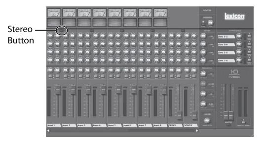
4. Turn the **Input 1 Pan** knob (just above the **Mute** button) to the 12 o'clock position (C).
