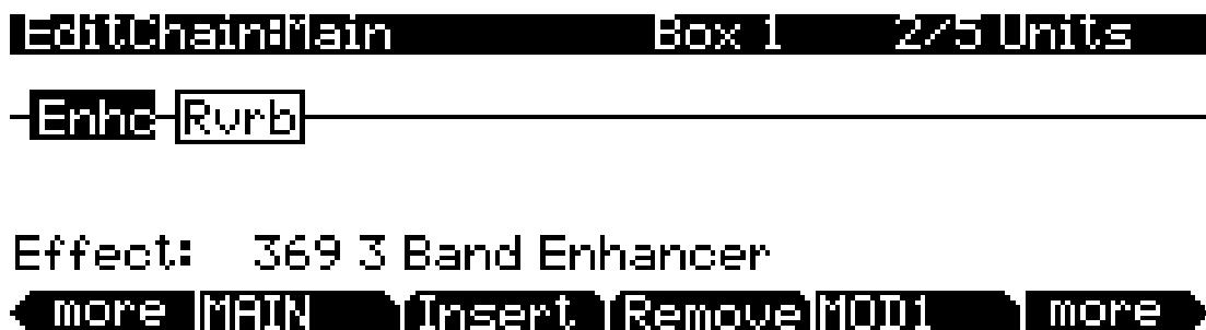
At the top right of the display is the number of DSP units used by the currently selected effect-box, and by the Chain as a whole. **2/5 Units** indicates that the current effect-box is using two DSP units and the Chain is using a total of five DSP units for all of its effects. There are a total of 16 units available for all of the Chains that are currently loaded by programs and any active Aux overrides from Setup/Song/Effects mode.
