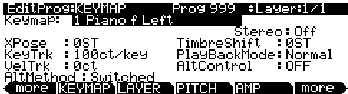
The top line of the display gives you the usual reminder of your location. It also tells you which layer you're viewing, and how many layers there are in the program. You can use the **Chan/Layer** buttons to scroll through the layers, if the program has more than one.
